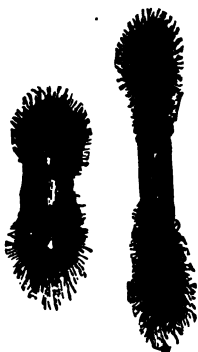
FIG. 89. A bar magnet dipped in iron filings. It is shaped like a bar. The ends of a magnet are called its poles.
